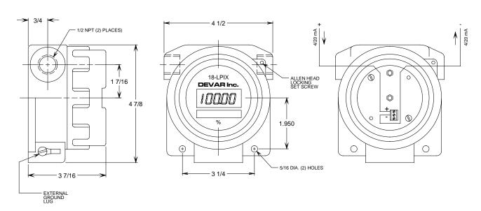
FIG. 1 GENERAL DIMENSIONS AND FIELD WIRING
